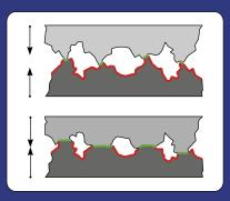
Above: Top section shows a low compression connection. Lower section shows the deformation of the plug and socket when compressed together. This compression displaces the soft tarnish as well as increasing the contact area.
